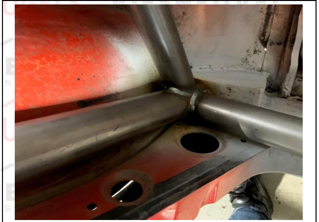
PHOTO 4 MAIN ROLLBAR TO FLOOR ATTACHMENT
