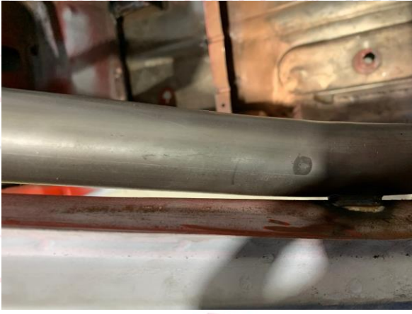
PHOTO 7 FRONT ROLLBAR TO "A" PILLAR ATTACHMENT
